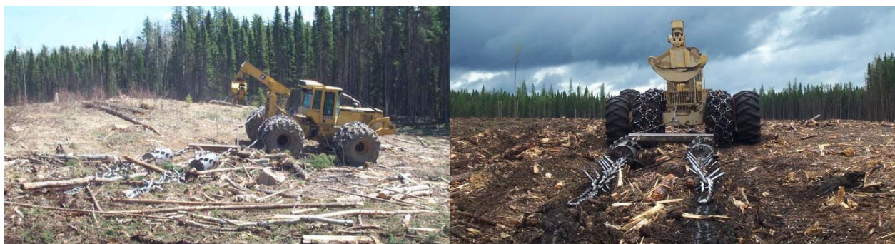
Figure 2.28 Scarification with barrels and chains
