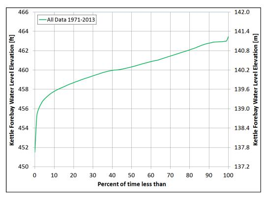
Figure 4-22: Kettle Forebay Daily Water Level Duration Curve
