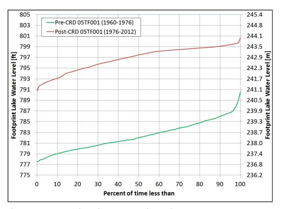
**Figure 4-19: Footprint Lake Water Level Duration Curve**
