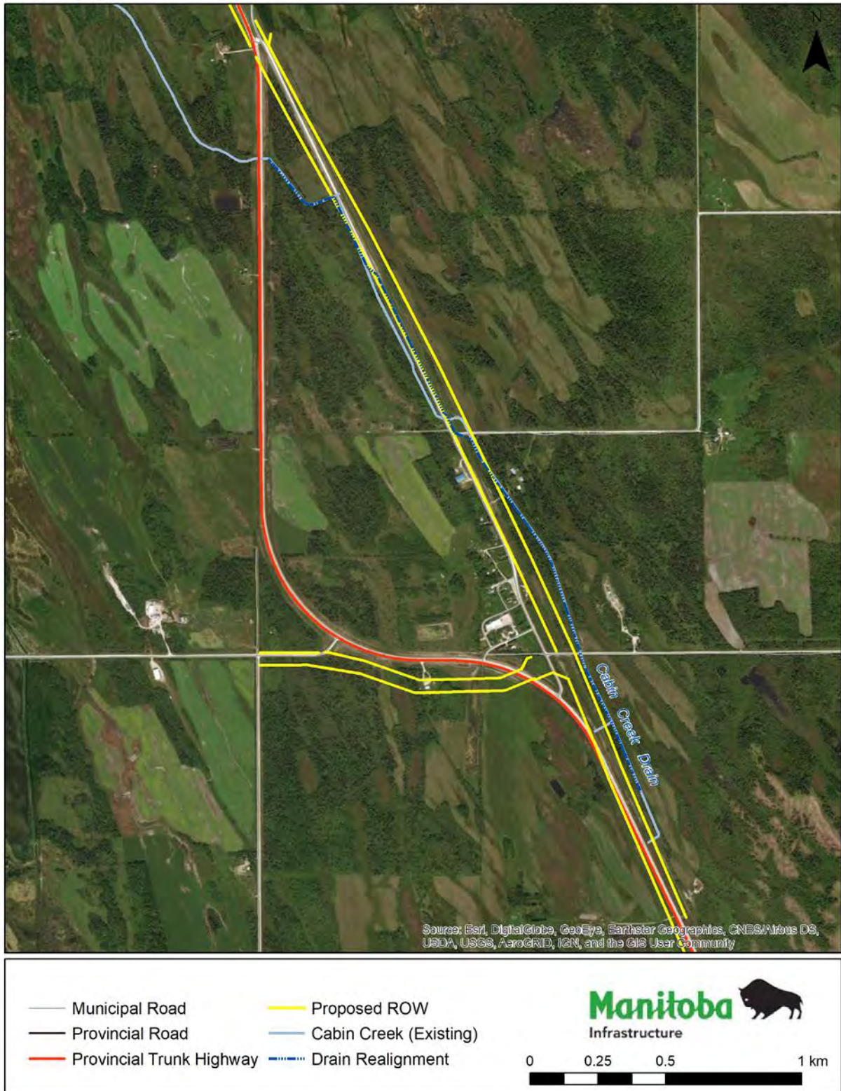
Figure 11 Relocation of Cabin Creek Drain Alignment
