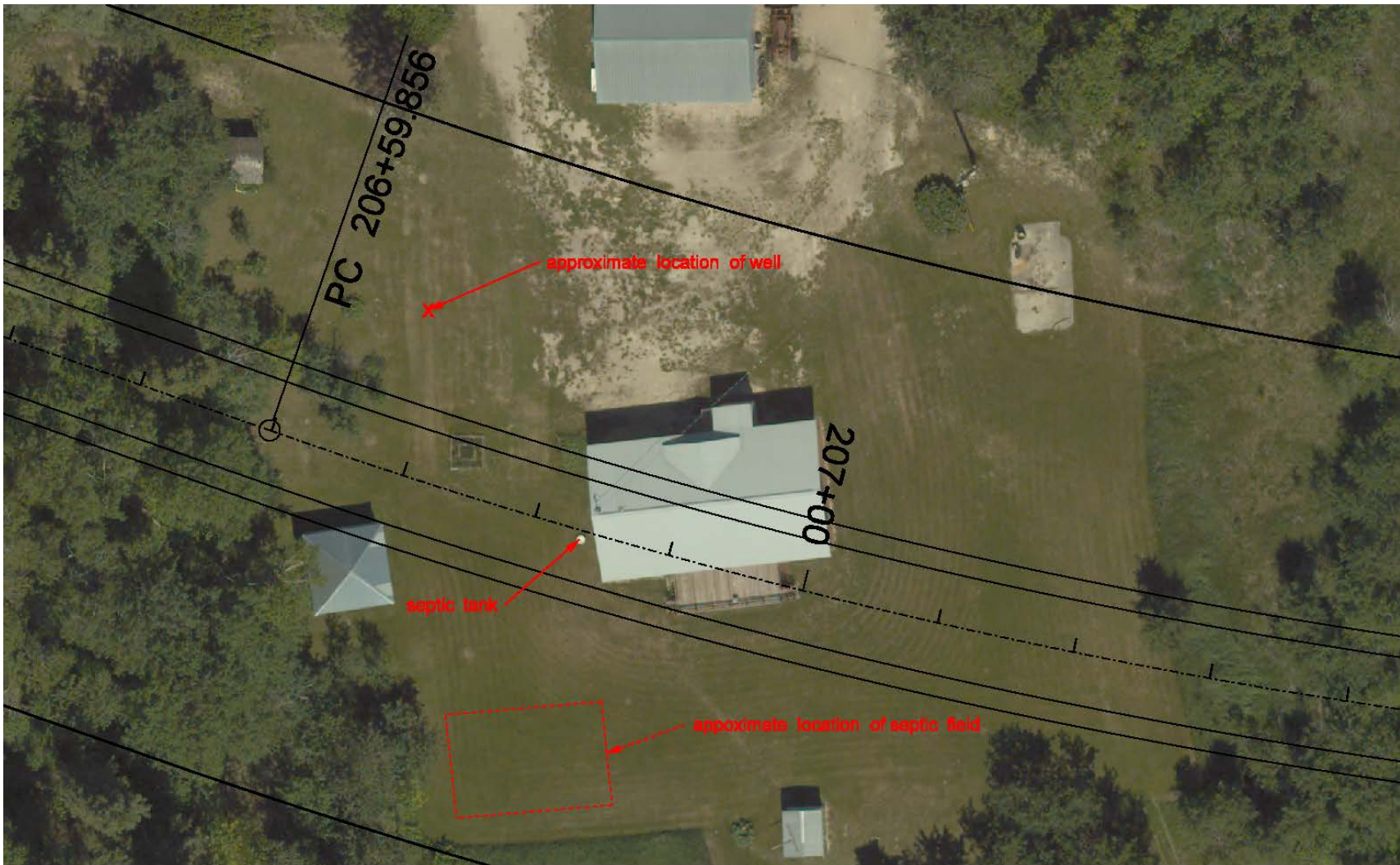
Figure 10 Realigned portion of Carne Ridge Road in relation to landowner Septic Field, Septic Tank and Groundwater Well
