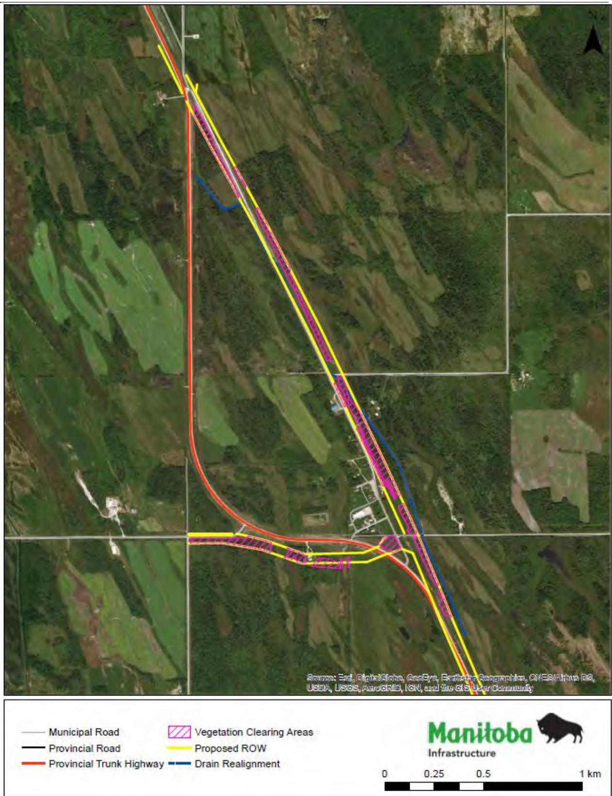
Figure 15 Project Areas that Require Clearing
