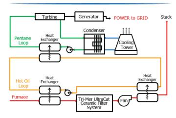
The Tri-Mer System presents the optimal combination for pollution control performance and electrical power generation.
