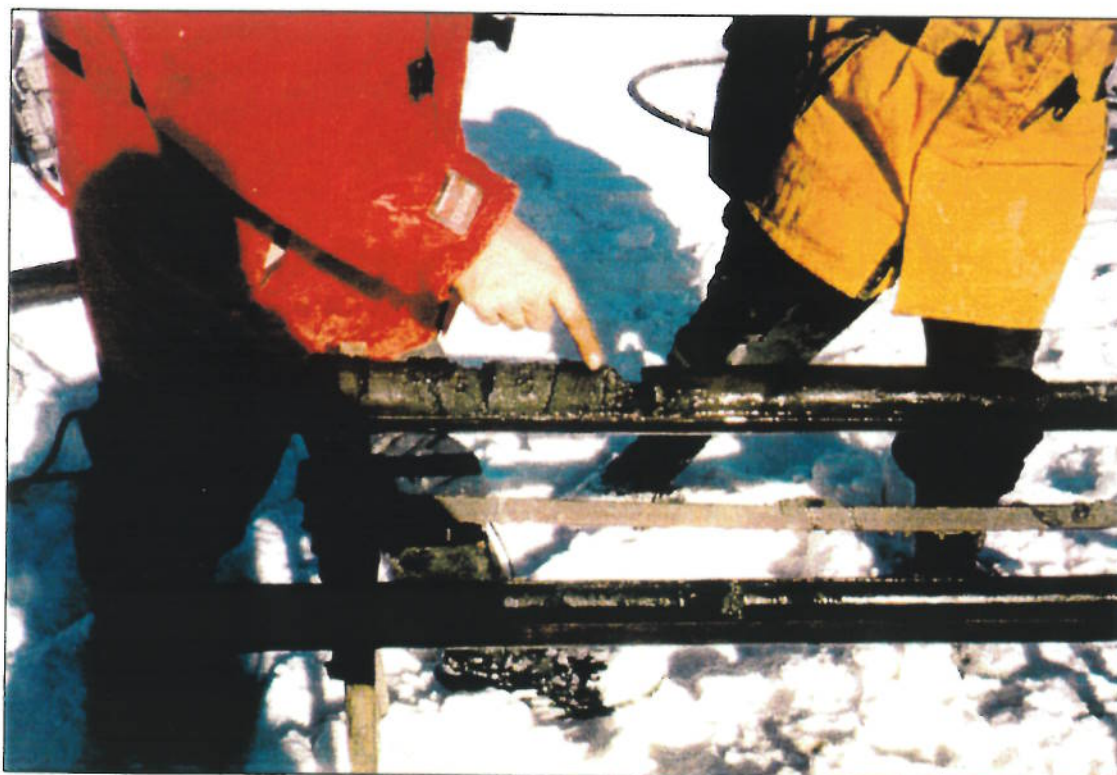
PHOTOGRAPH 4: VIEW OF LIQUID PHASE HYDROCARBONS IN A SAND LENSE IN BH01-28. NOTE BLACK PLASTIC COAL TAR IN SILT AND SAND AT THE RIGHT END OF THE SAMPLE.
