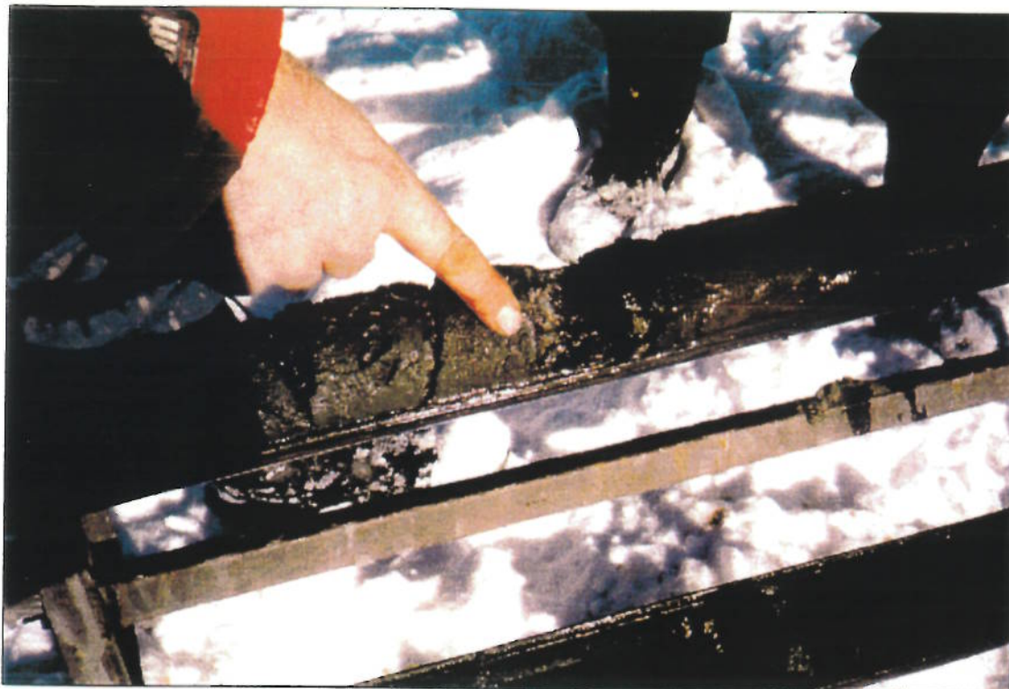
PHOTOGRAPH 3: VIEW OF LIQUID PHASE HYDROCARBONS AND HYDROCARBON SHEEN IN A SAND LENSE IN BH01-28.
