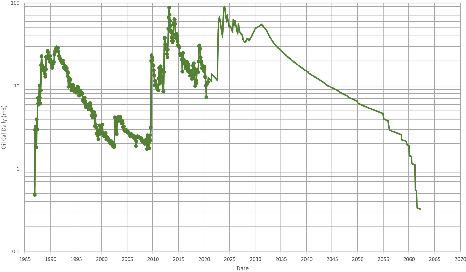
North Ebor 3 Waterflood Production
