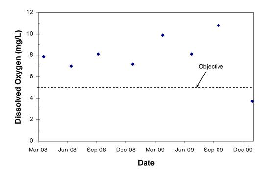
Figure 4: Dissolved Oxygen concentrations between 2008 and 2010 at the long-term water quality monitoring station in Willow Creek at Highway #8.
