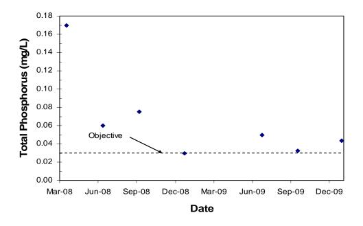
Figure 2: Total phosphorus concentrations between 2008 and 2010 at the long-term water quality monitoring station in Willow Creek at Highway #8.
