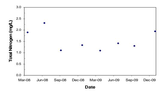
Figure 3: Total nitrogen concentrations between 2008 and 2010 at the long-term water quality monitoring station in Willow Creek at Highway #8.
